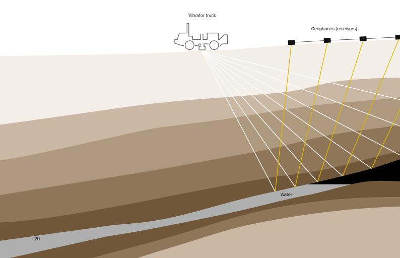
behind seismic is that sound waves travel at different speeds in different materials and that the sound waves, at the transition between different materials, partly bend and reflect back to the surface. As rocks have different compositions, it is possible, based on variations in the speed of the sound wave and angle, to estimate the location of structures that could hold oil and/or natural gas reserves in an exploration area.
