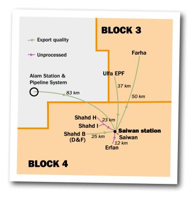
All production is transported through pipelines to the main exporting point at the Saiwan East facility. From Saiwan East, the oil is pumped through an 83 km long 16 inch pipeline to Alam Station just west of Blocks 3&4, for further transportation through the national pipeline system to the export port in Muscat, the Mina Al Fahal Terminal.
